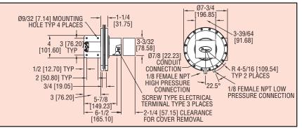
Our highest precision conventional large diaphragm pressure switch provides maximum dependability. In addition, it incorporates a visible set point indicator for maximum convenience. UL and CSA listed, FM approved for general service, these switches are suitable for most applications in air conditioning and industrial service. Electrical capability of 15 amps handles most small electrical loads.
