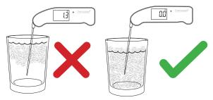
\*\* An improperly made ice bath can be off at the ice point by as much as 8 °C. See above illustration.
