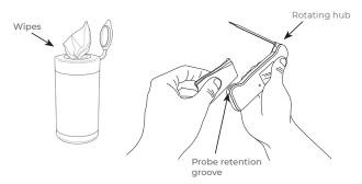
Proper cleaning after each use will prolong the life of your Thermapen and help keep you safe from harmful bacteria. Note that Biomaster silver ion technology is moulded directly into the plastic housing of the Thermapen ONE to help reduce microbial growth.
