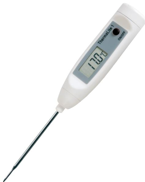
**INSTRUMENT OPERATION** - The instrument is switched on by pressing the ON/OFF button located on the front of the thermometer. Insert the probe into the substance being measured. The instrument reading may take a few seconds to stabilise, depending on the nature of the measurement. The instrument will automatically turn off after 10 minutes.
