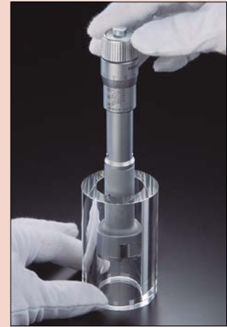
Constant-force device ensures repeatable measurement.
